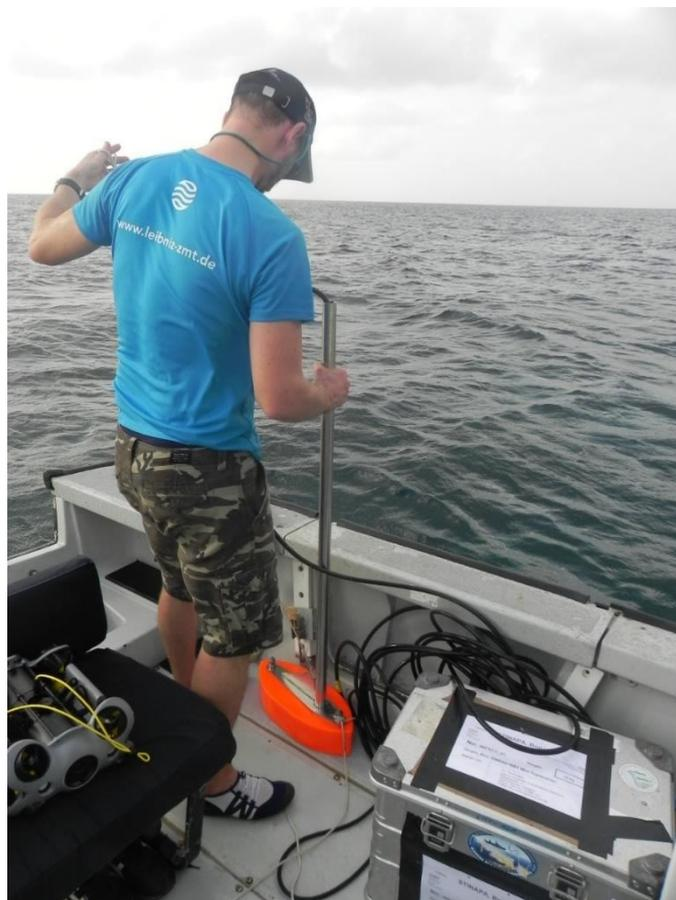
Figure 3. Transducer and pole being deployed on the STINAPA boat. Licensed under CC BY-SA 4.0.
