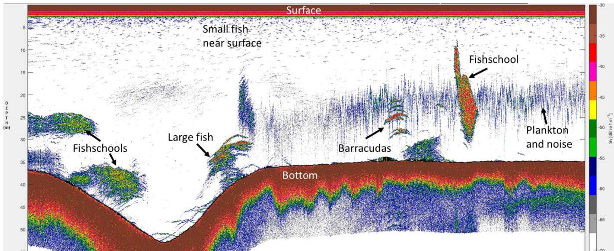
Figure 14. Echogram showing the multitude of fish signals in the water at Salt Pier station. Large fish can be clearly distinguished by the sickle shaped echoes from smaller fish and schools. Licensed under CC BY-SA 4.0.
