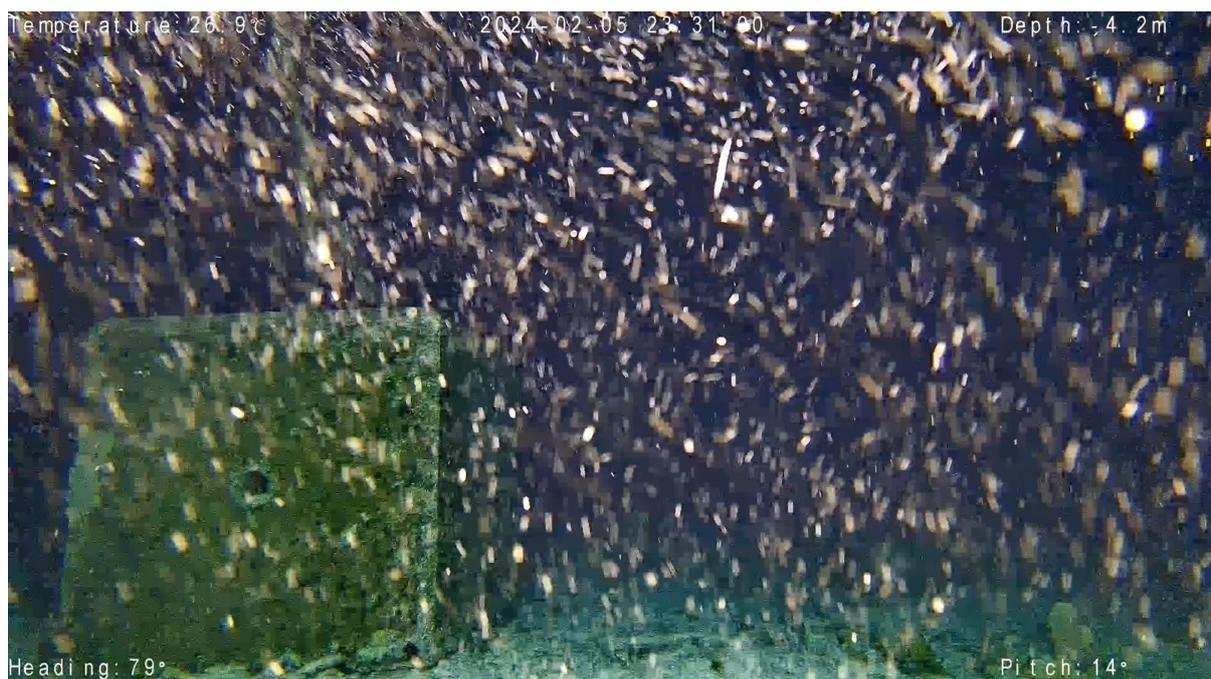
Figure 23. Swarms of plankton attracted by the ROV light almost obscure the presence of a mooring concrete block in a shallow water night test from the beach. Licensed under CC BY-SA 4.0.
