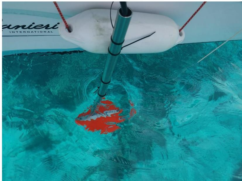
Figure 2. Transducer (orange) and pole mounted to the side of the boat. Licensed under CC BY-SA 4.0.
