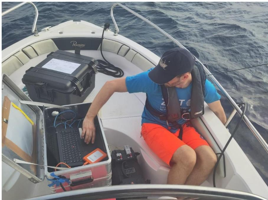
Figure 5. The signal from the hydroacoustic transducer deployed in the water is being checked in real time on the laptop housed in the Zarges box. The battery casing is visible next to it. Licensed under CC BY-SA 4.0.
