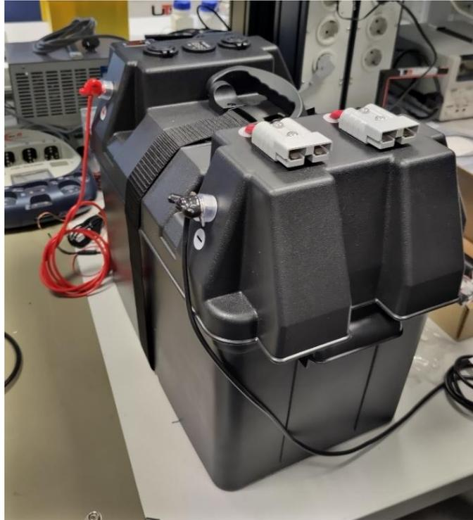
Figure 4. Customised travel case for the battery used to provide a constant power source onboard for the hydroacoustic tool. Licensed under CC BY-SA 4.0.
