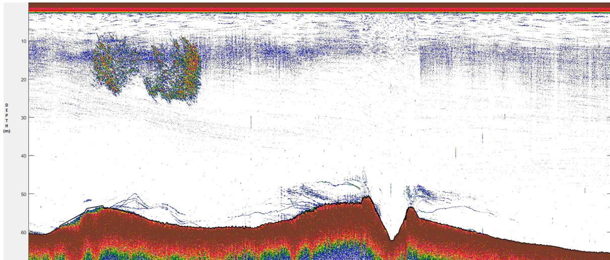
Figure 21. Echogram at low speed showing pelagic fish schools as well as individual fish at the bottom between 50 and 60m depth. Note: Each line is the trajectory of a single fish near the bottom. Licensed under CC BY-SA 4.0.
