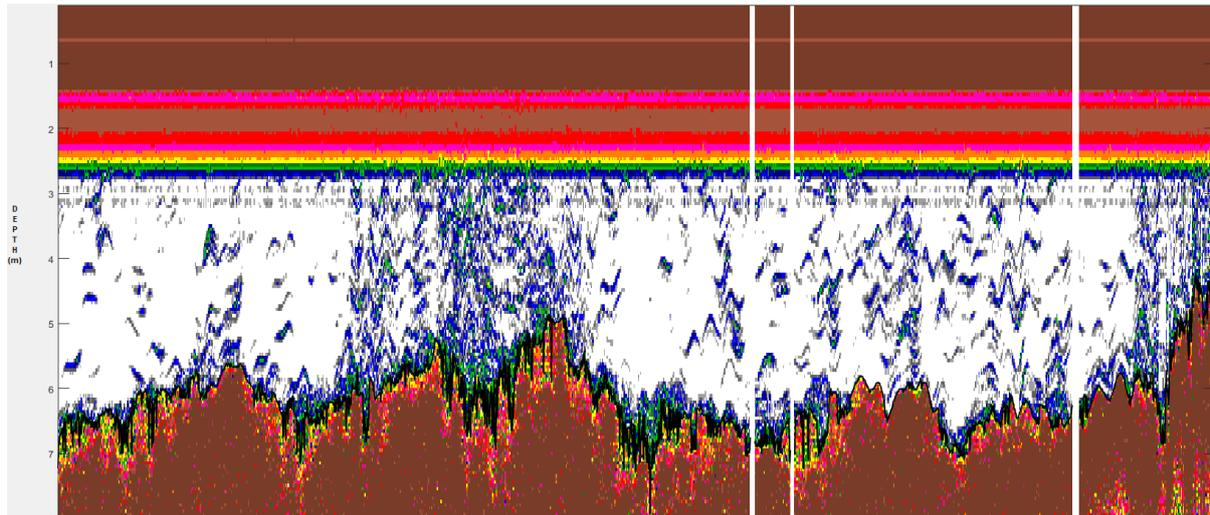
Figure 13. 38 kHz echogram showing individual small fish (blue shapes) and fish groups at shallow depths of 6m. Notice the black, thin line representing the detected bottom, the white vertical lines indicating removed pings (no data) and the acoustic surface deadzone (horizontal red and pink stripes) up to 2.8m depth. Licensed under CC BY-SA 4.0.
